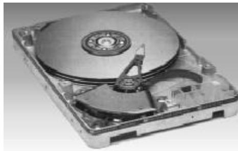
Usually (as in the picture above) several physical disks are contained in one harddisk unit. Each disk is known as a **platter**. Typical hard disk capacities for a home PC now start at up to 180 Gb.
