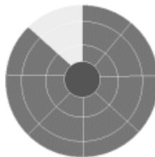
**Double side** - A typical magnetic disk has two surfaces or sides. Each surface holds data in circular tracks and each track is divided into equal sections called sectors. The track number and sector number are used as an address to find where data is on the disk. Data can be **both written to and read from** the disk. Magnetic disks are **direct access** i.e. any data item can be accessed without reading other data first.
