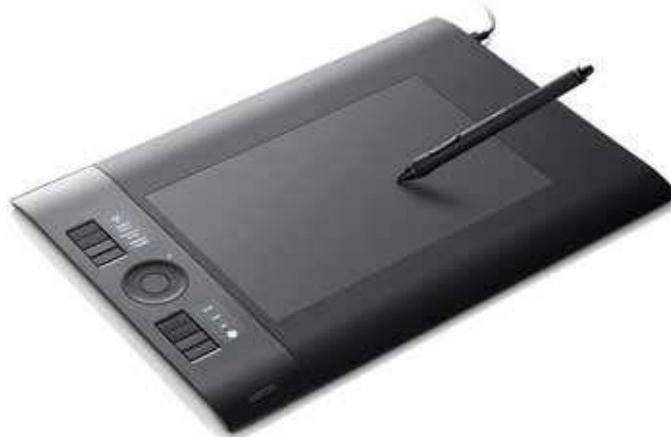
Digitizer is also known as Tablet or Graphics Tablet as it converts graphics and pictorial data into binary inputs. A graphic tablet as digitizer is used for fine works of drawing and image manipulation applications.
