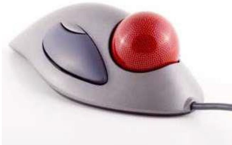
Since the whole device is not moved, a track ball requires less space than a mouse. A track ball comes in various shapes like a ball, a button, or a square.
