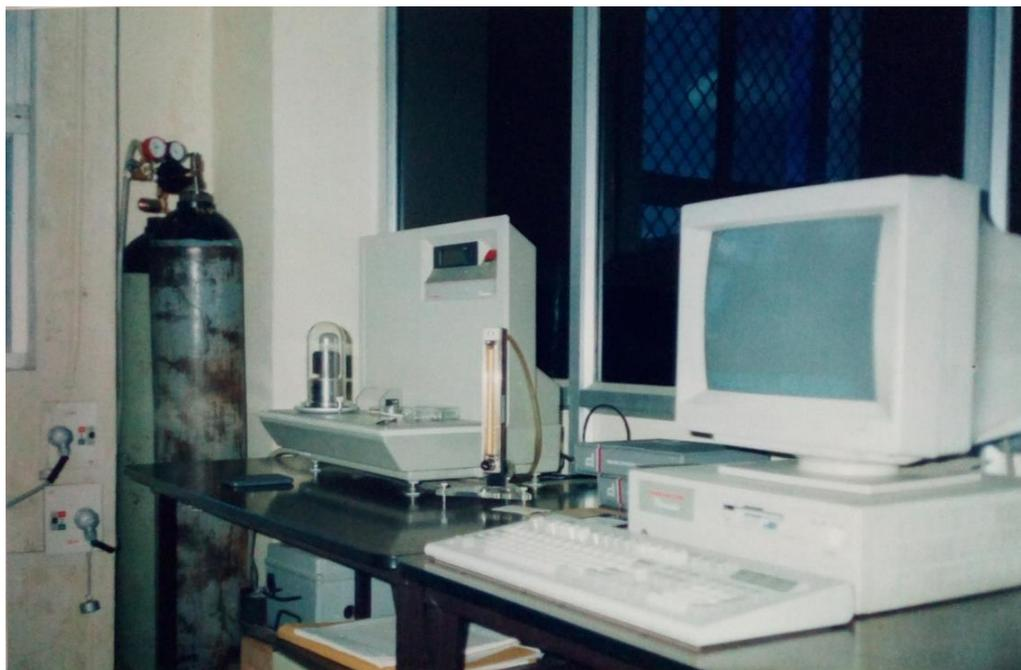
Fig. 2.6: A picture of DSC 2910 (TA Instrument Inc. USA) system
